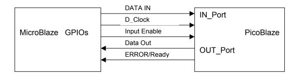
*Figure 6:* MicroBlaze – PicoBlaze Bit Serial Interface
