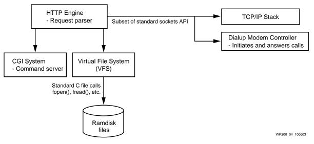
Figure 5: HTTP Engine Task
