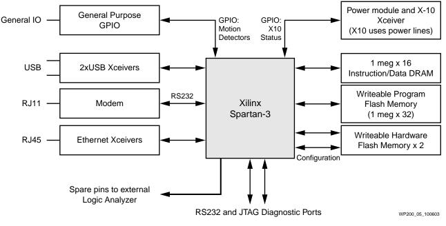
Figure 2: Block Diagram of the System Board
